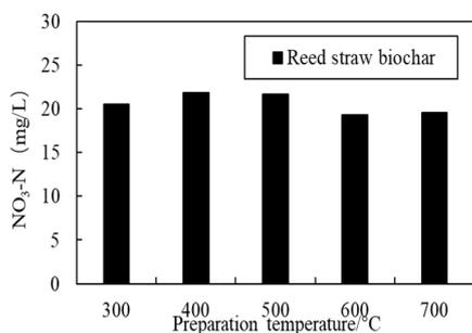
Figure 1: Adsorption effect of reed straw biochar prepared at different temperatures for NO<sub>3</sub>-N.
