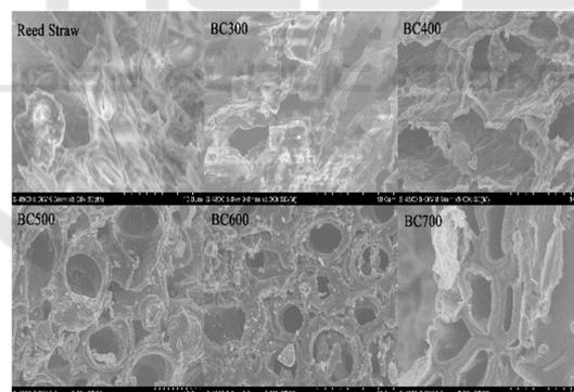
Figure 2: Micro-morphology pictures of SEM (10 μm) prepared by biochar at different temperatures.
