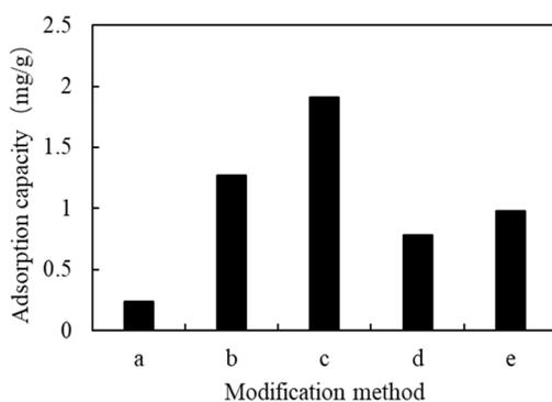
Figure 3: Adsorption effect of NO<sub>3</sub>-N on biochar under different modified methods.
