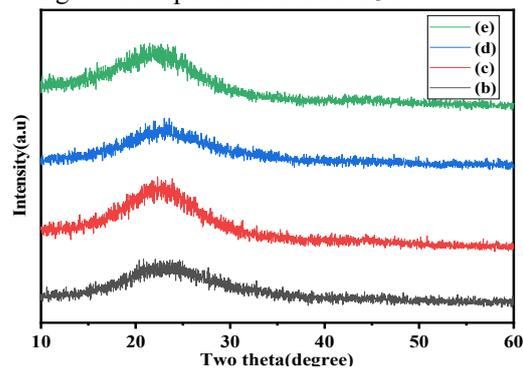
Figure 5: XRD pattern of biochar modified by FeCl<sub>3</sub> solution.
