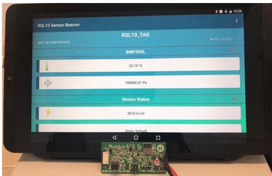
Figure 7: The connected object that send data to the tablet application.
