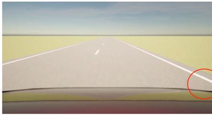
Figure 5: In this case, the vehicle is positioned to the left of the desired lateral position. Looking at the red circle, which indicates the position of the right lane boundary with respect to the vehicle, helps to see this. See Figure 4 for comparison. This is the behaviour which is received when the vehicle has been trained with perfect steering mechanics, and an offset is added to the steering angle during the inference phase.
