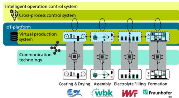
Figure 1: ViPro overall system architecture.
