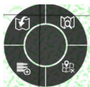
Figure 5: The context sensitive menu for a given tactical position displaying four icons for the following actions: occupy area, identify area, delete area, and reload launchers.
