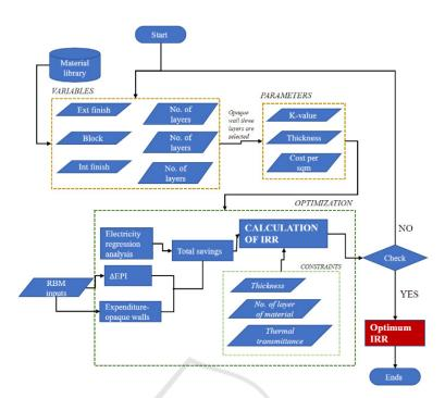
Figure 3: Optimization process flowchart.
