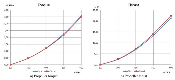
Figure 3: Comparison of the results of computer simulation and the results of model testing of propeller in test basin.
