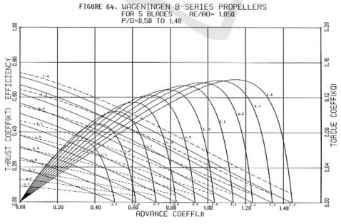
Figure 2: Performance curves of the propeller.
