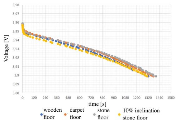
Figure 9: Robot-o on different floors with rubber footwear according to (Koren, 2021).
