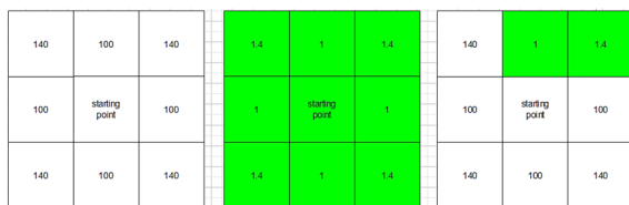
Figure 5: Different assignment of g(n) cost value to different pixel points.
