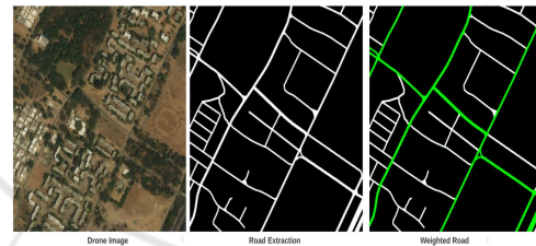
Figure 4: Road extraction, analysis, and marking of green priority roads.
