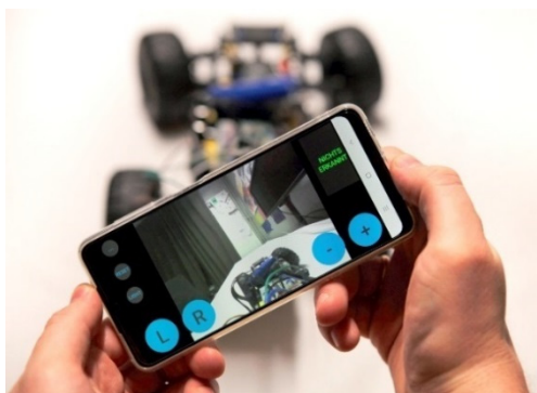
Figure 4: App usage to control the car via sensor.
