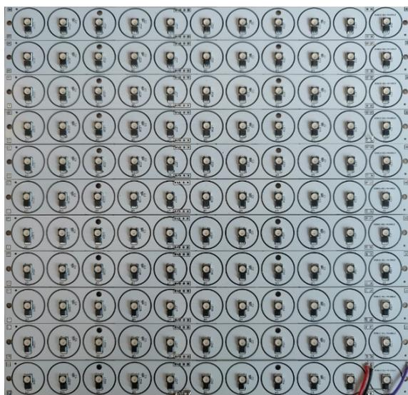
Figure 4: LED and sensor Matrix.
