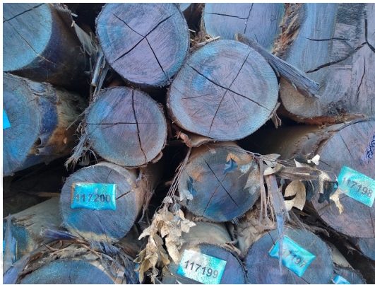
Figure 2: Cracks in wood logs.
