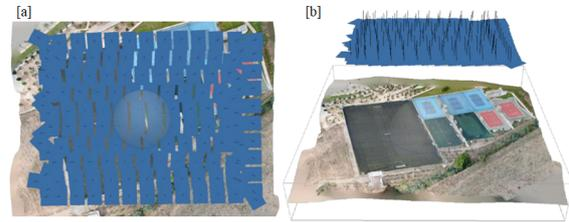
Figure 6: Image processing, where: (a) Distribution of images collected to cover the AOI, and (b) 3D model extraction of the AOI.
