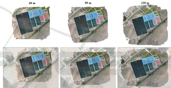
Figure 7: Resulted orthophotos for each altitude flight compared to the respect scene of Google satellite basemap.
