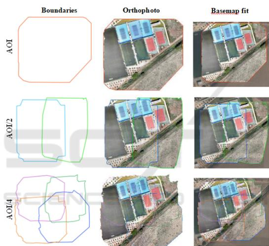
Figure 8: Resulted orthophotos for each flight with different AOI boundaries, compared to the respect scene of Google satellite basemap.
