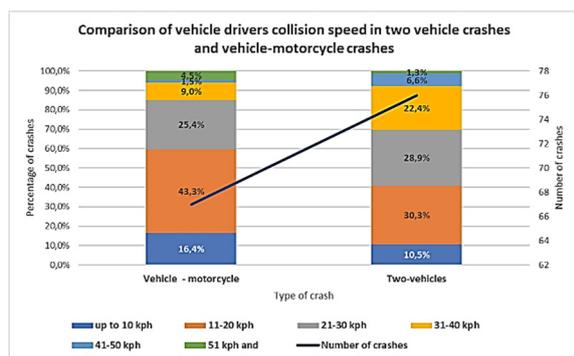
Figure 3: Comparison of vehicle driver’s (who failed to give way) pre-collision speed in two vehicle crashes and vehicle-motorcycle crashes.
