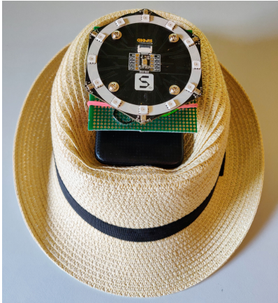
Figure 2: Portability of the hardware used for sound direction detection.
