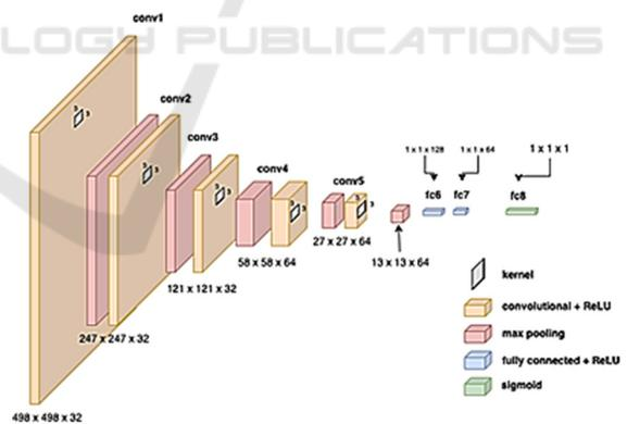
Figure 3: Consolidated architecture of the CNN with the display of parameters at each level.
