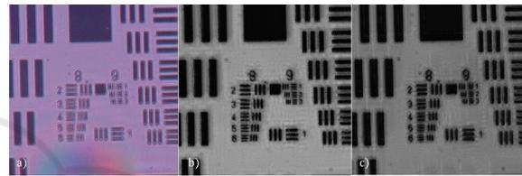
Figure 3: a) Original image captured with central LED, b) Reconstructed image without applying focus adjustment c) Reconstructed image with focus adjustment.
