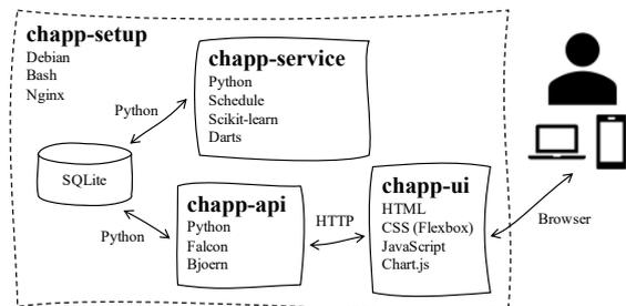
Figure 6: Software architecture.
