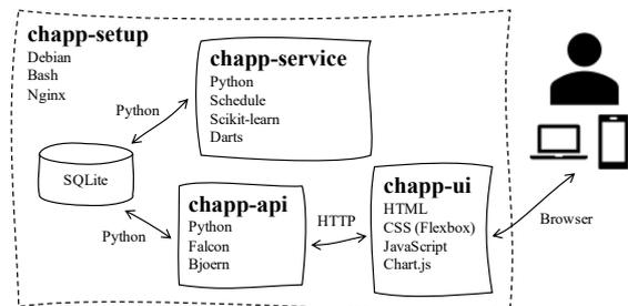
Figure 6: Software architecture.
