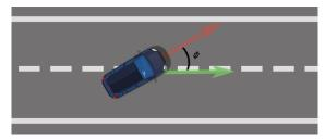
Figure 2: Angle  $\phi$  between agent vehicle moving direction and road direction. While  $|\phi|$  is greater than  $\phi_{max}$ , steering towards the direction that further increases the angle results in a penalty.
