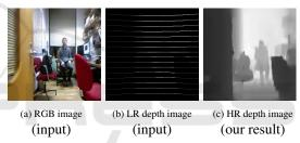
Figure 1: High resolution depth image generated from lowresolution depth image of LiDAR by using our proposed method. The low-resolution depth image is considered as defect image with holes and image inpainting is conducted for obtaining high resolution depth image with the proposed method.
