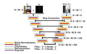
Figure 3: Generator of Proposed method 1.
