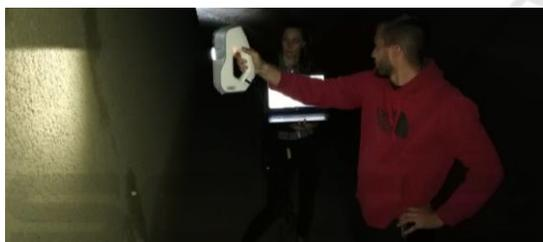
Figure 7: Scanning of test surface using Artec Eva.
