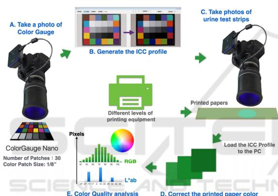
Figure 1: The experimental setup of the 2D chroma meter for the measurement of printed papers.
