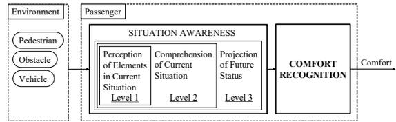
Figure 1: Process of passenger's comfort recognition based on the situation awareness.
