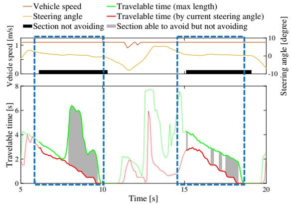
Figure 14: Sections where the vehicle is not avoiding and the sections where the vehicle is able to avoid but not avoiding (Scene No. 1).
