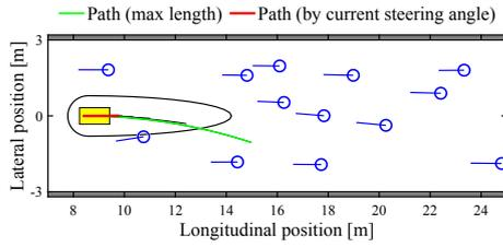
Figure 13: Difference in the length of the path that can be drawn by different steering angles (Scene No. 1).
