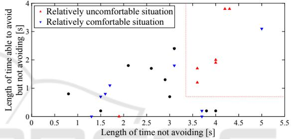
Figure 15: Classification based on the length of time that the vehicle is not avoiding and the length of time that the vehicle is able to avoid but not avoiding.
