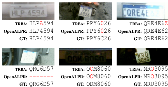
Figure 6: Some LP images from RodoSol-ALPR along with the predictions returned by TRBA and OpenALPR. Observe that one character may become very similar to another due to factors such as blur, low/high exposure, rotations, occlusions. For correctness, we checked if the ground truth (GT) matched the vehicle make and model on the National Traffic Department of Brazil (DENATRAN) database.
