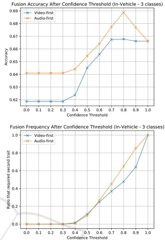
Figure 9: Cascade results in the in-vehicle scenario with 3 classes: overall classification accuracy (top) and fraction of instances that need the secondary modality (bottom) for different confidence thresholds.
