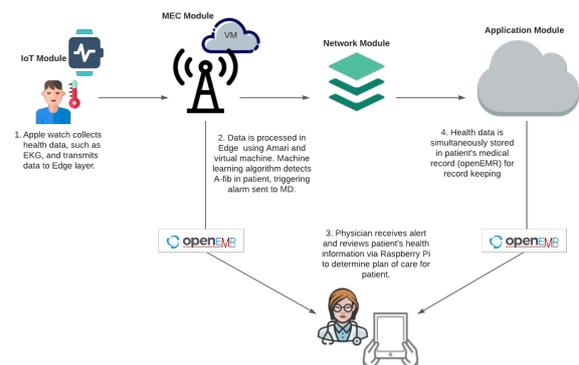
Figure 3: System Component Connection.
