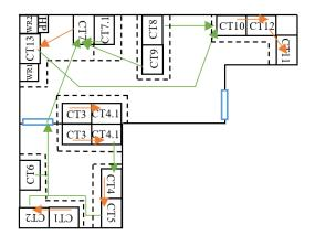
Figure 6: ICP production line layout resulting from the SLP approach.
