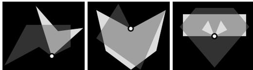
Figure 2: Example pairs of objects unsupported by the current 2D vector  $\phi$ -descriptor algorithm. Each of these feature polynodes that map to more than two  $\phi$ -regions directly above them. The relevant polynodes have been marked.
