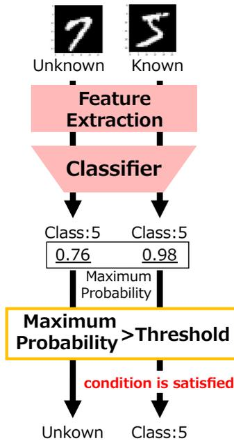
Figure 2: Block diagram of discriminative model-based methods.
