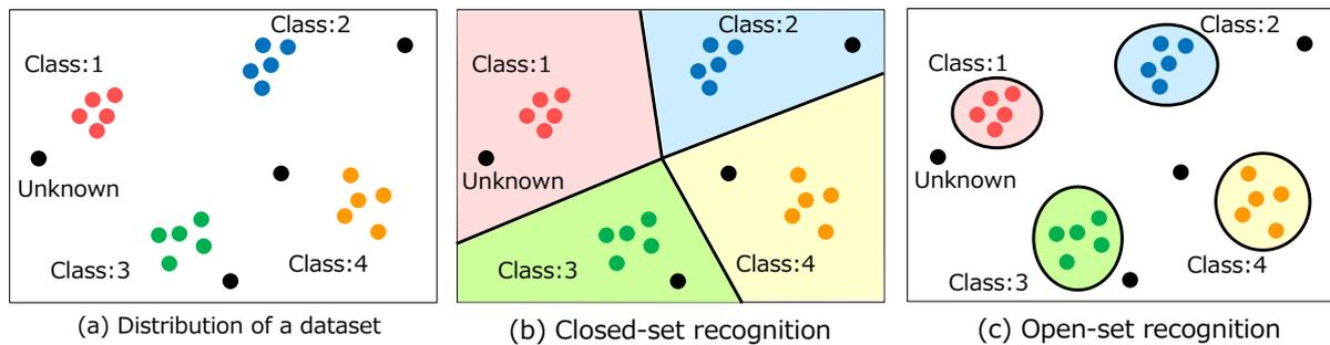
Figure 1: Comparison of closed-set recognition and open-set recognition.
