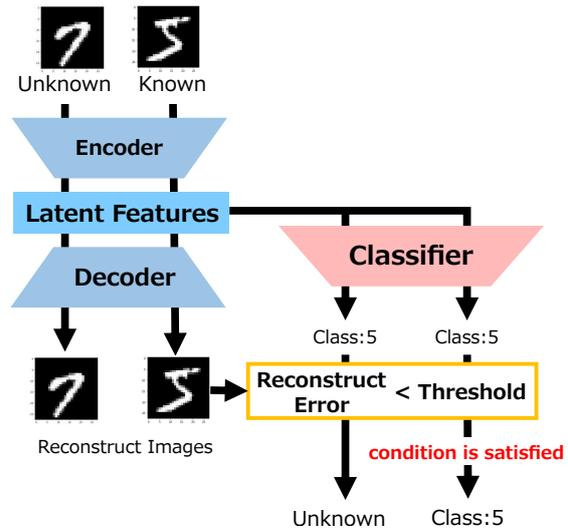
Figure 3: Block diagram of reconstructive model-based methods.
