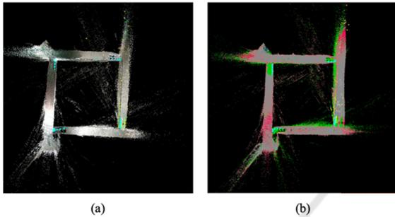
Figure 10: Output with loop closure detection: (a) pre-existent RTAB-Map, (b) RTAB-Map output labeled with a semantic segmentation output image.
