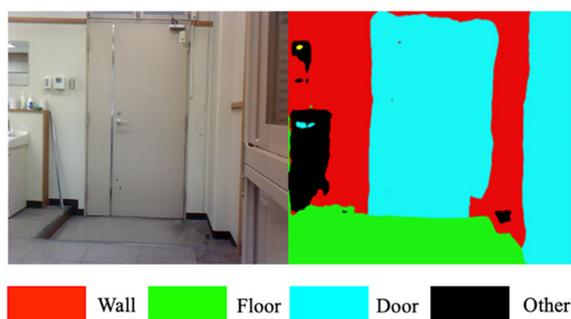
Figure 1: Identifying a floor with a step as a continuous single-level domain.
