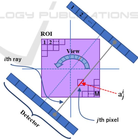
Figure 1: The discretized model of the image reconstruction problem.
