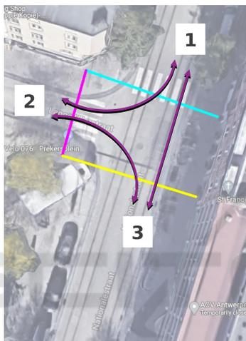
Figure 3: Lines defined for automatic turning movement counting. Arrows show the possible vehicle movements excluding u-turns. Map Data: ©2021 Google, ©2021 Aero-data International Surveys.
