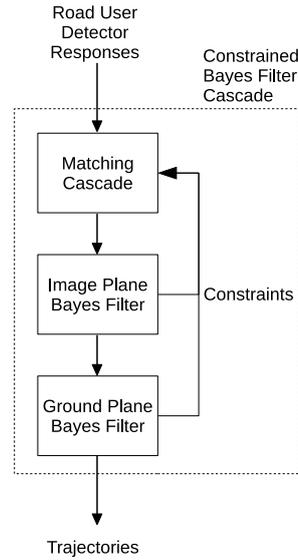
Figure 1: Modules of the proposed Bayes filter cascade.
