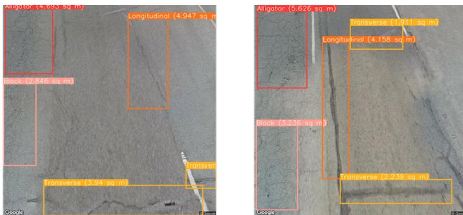
Figure 7: Example model outputs showing the real-world measurements for distress regions in square meters. Pavement images were obtained from Google Street View panorama using a pitch of  $-70^\circ$  and FOV of  $90^\circ$ .
