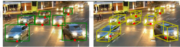
Figure 1: Localization using 2D and 3D bounding boxes. Note the difference between the estimated ground-plane location (red dot) for both bounding boxes.
