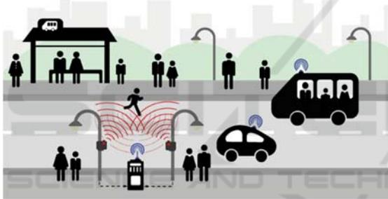
Figure 1: Radar sensors, locating on the opposite side of the road, detects a pedestrian, which is leaving the static group while crossing the street. Car2X message is sent out from central unit to warn the surrounding traffic.
