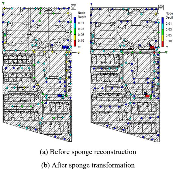
Figure 6: Distribution of simulated node water depth during rainfall process on August 3, 2019 ( the maximum water occurred at 3:10 ).
