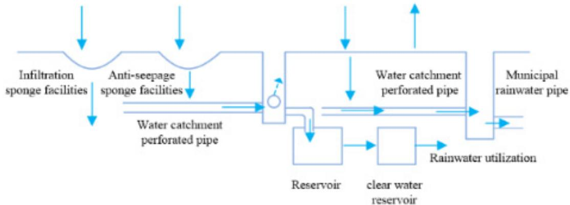
Figure 1: Diagram of the process of rainwater runoff control in the sponge transformation community.
