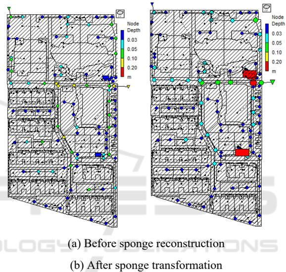
Figure 7: Water depth distribution of simulated nodes during rainfall on 27 June 2019 ( the maximum water occurred at 6:15 ).
