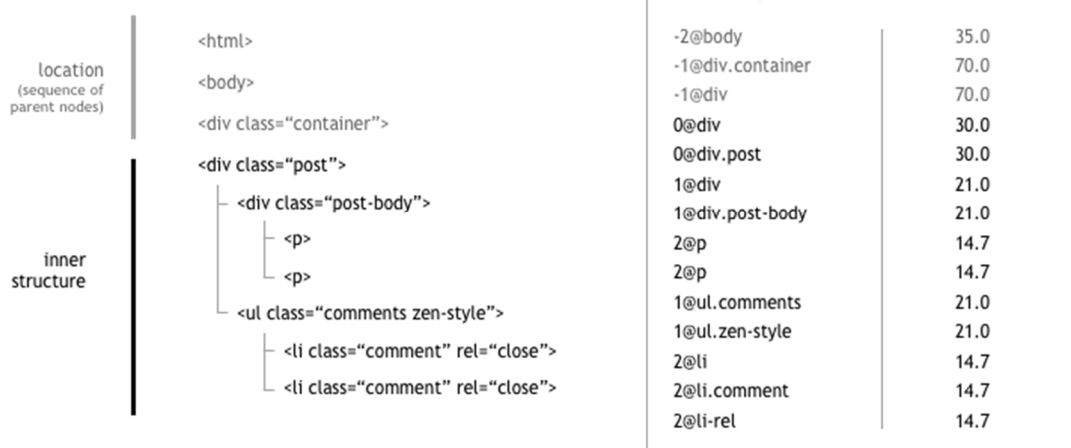
Figure 1: Sample DOM Element and its corresponding comparison map.
