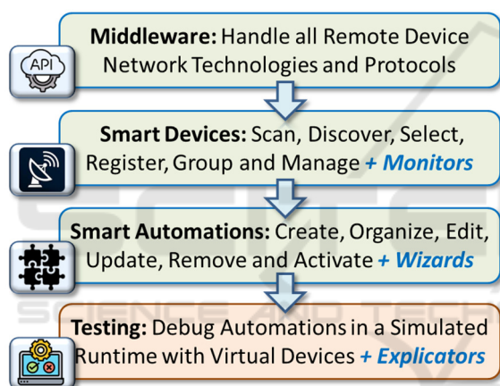
Figure 2: End-user tool layers required to enable crafting of personalized smart automations (from Savidis, 2021).
