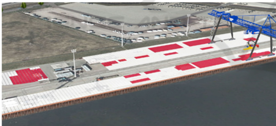
Figure 4: 3D model of the Hanse-Terminal with Virtual Storage Location Grid (occupied locations marked red).
