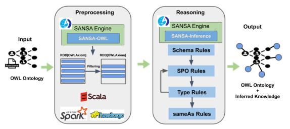
Figure 2: The architecture of the proposed approach.
