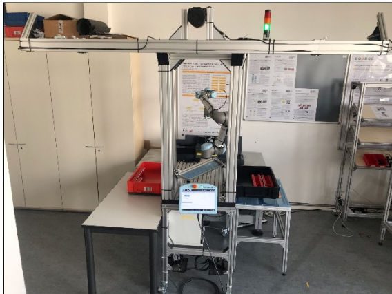
Figure 1: Flexible and mobile robotic cell.
