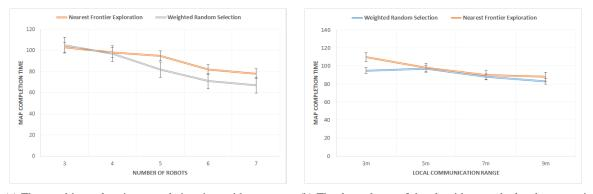
(a) The trend in exploration completion time with respect to (b) The dependence of the algorithms to the local communithe number of robots. (Local communication range = 5m) cation range. (For five robot fleet)
