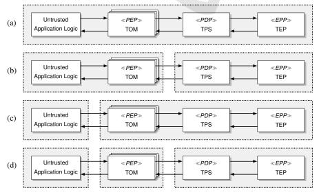
Figure 2: APPSPEAR instantiations with different separation/isolation of the architecture components.
