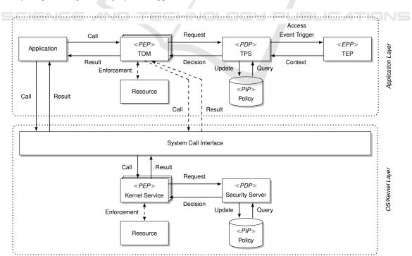
Figure 1: Functional architecture for mutually independent policy enforcement on application layer (APPSPEAR) and OS layer (SELinux/Flask).
