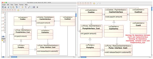
Figure 7: The gas station specification in Metaedit+.
