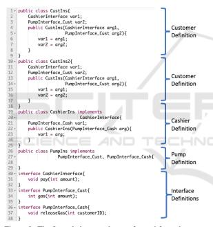
Figure 9: The Java skeleton code transformed from the gas station specification in Metaedit+.
