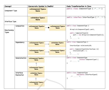
Figure 5: Mapping pattern definition concepts with DesPat's meta-model (concrete symbols and Java transformation).
