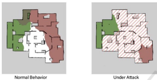
Figure 5: Map building in a scenario with and without attack.
