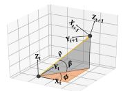
Figure 2: The relative translation expressed by two angles,  $\phi$  and  $\beta$ , and a scale factor  $\rho$ .
