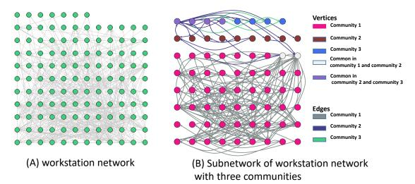
Figure 3: Visualization of (A) the workstation network and (B) the routing of three communities of materials identified by the biLouvain community detection algorithm.
