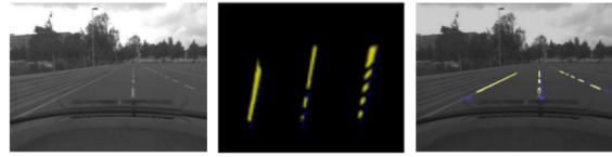
Figure 6: Examples of the camera lane detection. Left : Original rectified image. Center : Binary image in bird eye's view. The yellow points represents the segmented points and the blue points (centroids) are extracted by the sliding window algorithm. Right : The segmentation (yellow) and the centroids (blue) are augmented in the rectified image.
