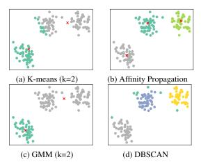
Figure 2: Effect of setting the wrong numer of clusters k for clustering with k-means and GMM, whereas DBSCAN and AP determine the number of clusters automatically. The red crosses mark the clusters' centroids in the respective clustering algorithm's output.
