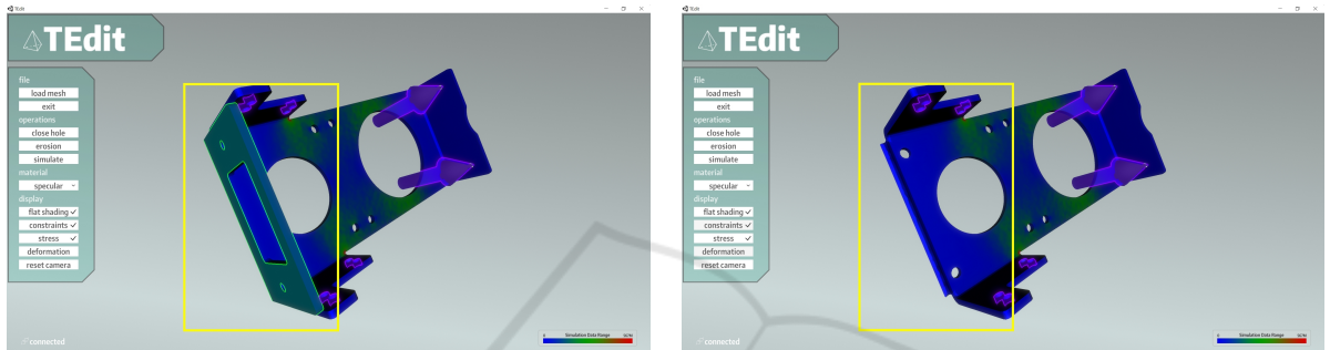
Figure 4: Von Mises stress before ( left ) and after ( right ) eroding the selected part of the model (highlighted in yellow). The model is part of the ABC dataset (Koch et al., 2019).
